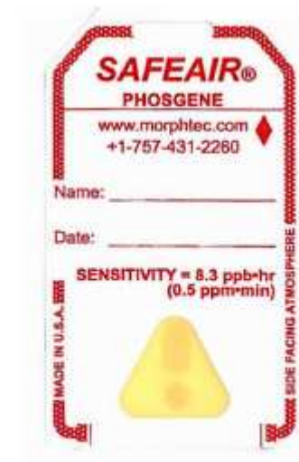
Figure 13. SafeAir Phosgene Dosimeter Badge 37
